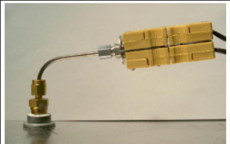
Figure 1-32 Dual Thermocouple Installed
