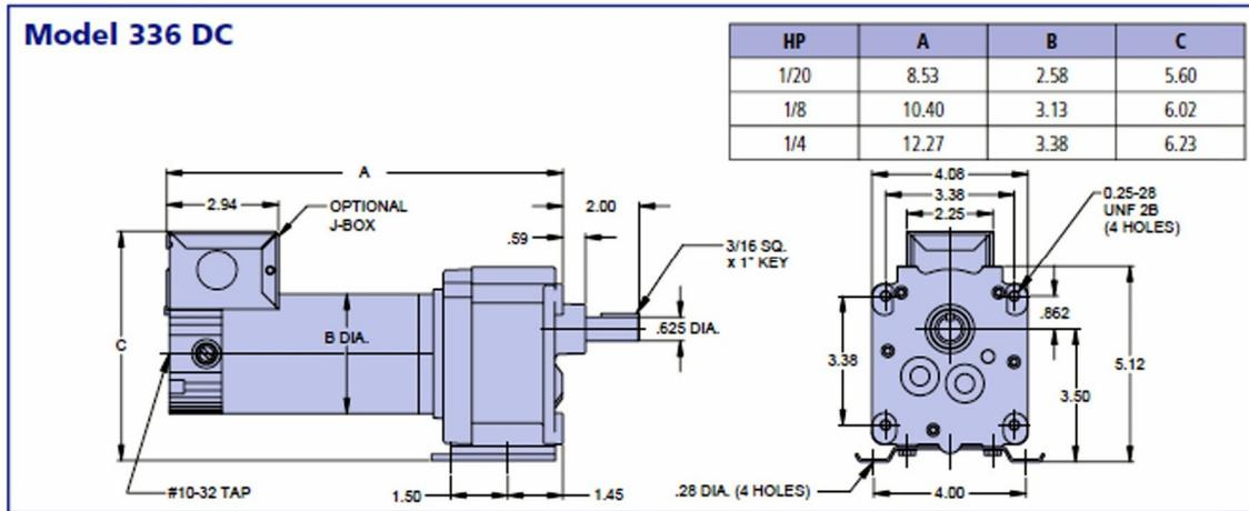
Figure 1-23 DC Drive Motor, Medium Speed
