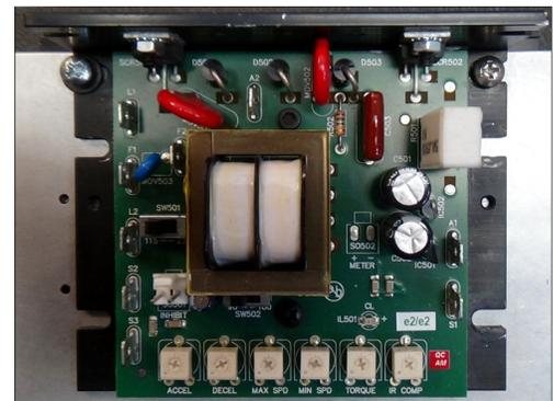
Figure 1-20 Motor Controller
