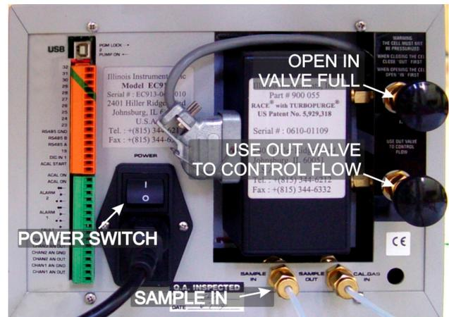
**Figure 1-39** EC913 Oxygen Analyzer Rear Controls
