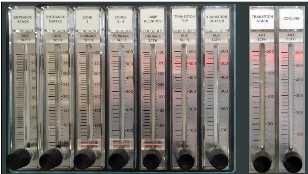
Figure 1-11 Gas Flowmeters - Dual Mode
