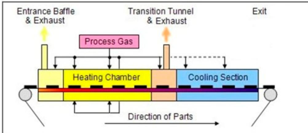
Figure 1-8 Process Sections
