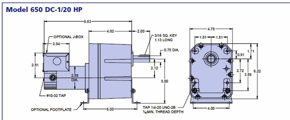
Figure 1-25 DC Drive Motor, Low Speed
