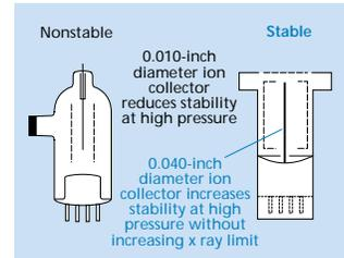
Ion space charge at high pressures must be minimized.
