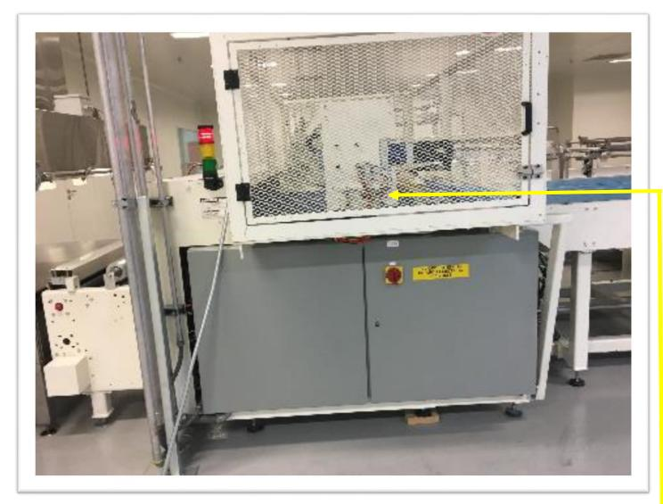
Picture 2b: Cutting machine with inlet accumulator. Knife with movement for maximum +/- 10 degrees cut angle
