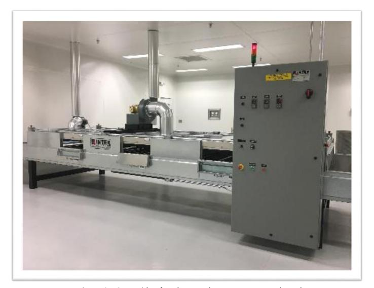
Picture 3a: Oven with safety doors, and temperature control panel.
