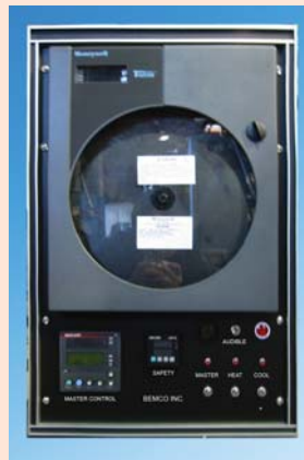
Bemco FTU3.2-184X538C with counterbalance stand and large window. This unit uses LN 2 for cooling.
