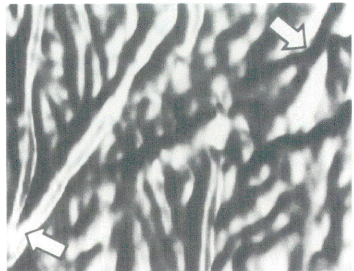
Light shaded AFM image of a cryomicrotomed surface of ultrahigh molecular weight polyethylene. The arrows indicate zones with lamellae splitting.
