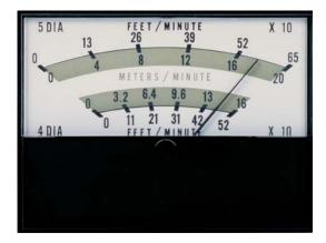
Tachometer display in surface feet-/ meters-per-minute
